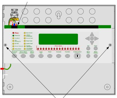
REMOVE FIXING SCREWS TO RELEASE PLATE AND PCB
