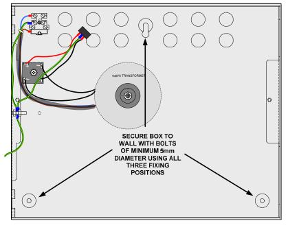
Remove knockouts from the top and or back of the box in the positions at which cables will enter.
